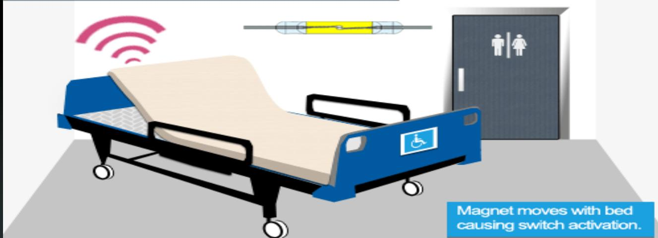
Magnet moves with bed causing switch activation.
